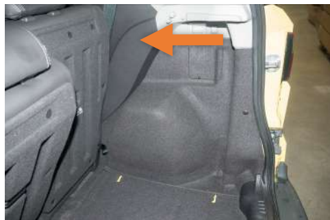
Offside - rear seats do not lock into D-Ring mounted onto plastic boot side
