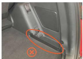
The cargo liner does not accommodate these separators, they need to be removed from the vehicle before fitting.
