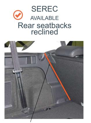
When the seats are most reclined there is no void between the seat upper and the plastic molding
