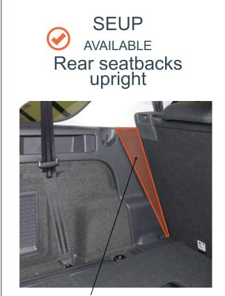
When the seats are most upright there is a void between the seat upper and the plastic molding
